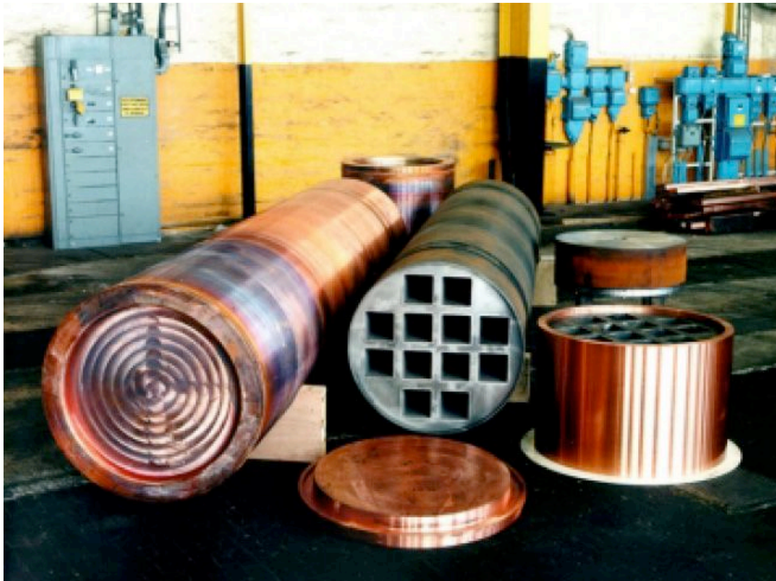
Figure 5.10: Copper-shell with steel insert disposal container parts
