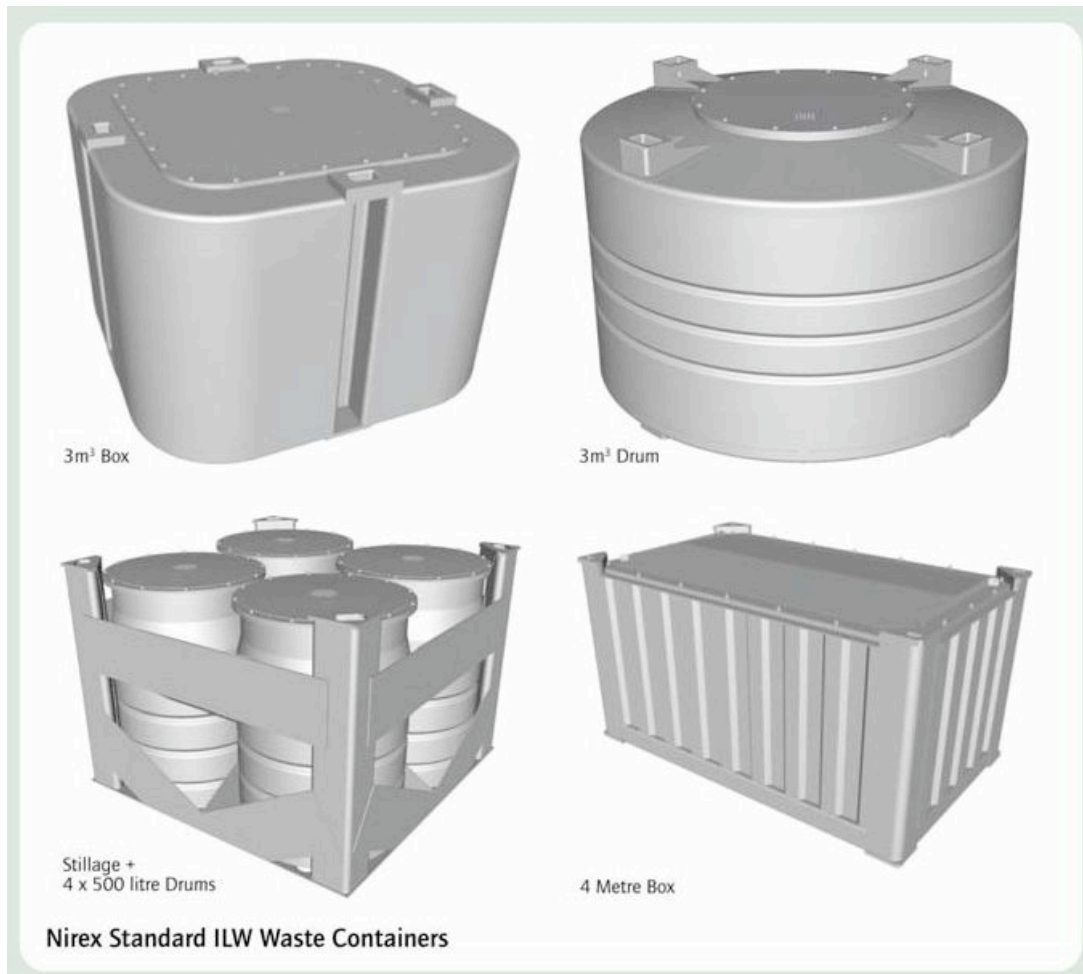
Figure 5.5: Standard ILW packages as specified in the UK (not to scale), from [48]
