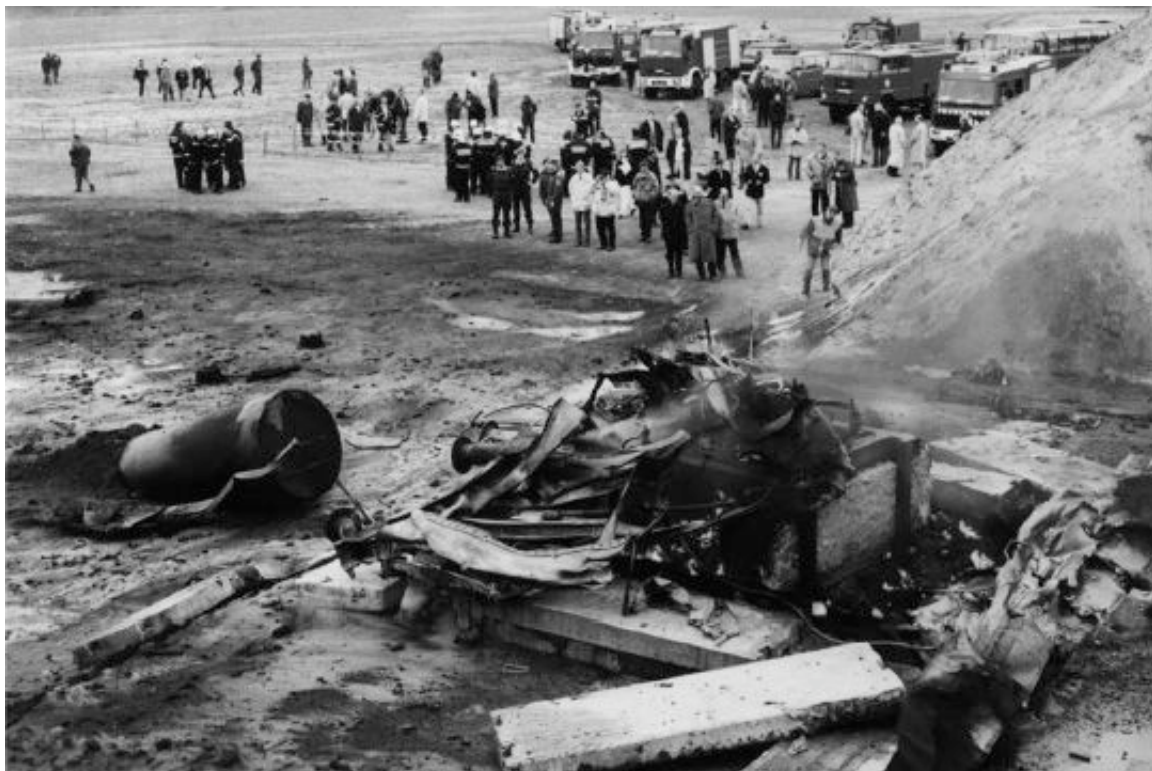
Figure 5.8: Post-explosion view of test of the impact of LPG container explosion (centre right) on a CASTOR SF container (left), from [51]
